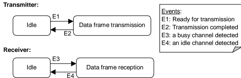
Figure 2.1: The finite state machine of an Aloha transceiver
